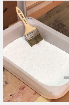
Fig. 5 Preparation of the water-plaster mixture
