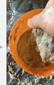
Fig. 9 Using the gypsum-paper cement for modelling
