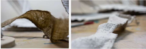
Fig. 1 Burlap stiffened with glue and with plaster.
